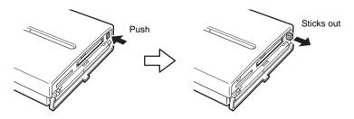
**2** Push the eject button all the way in, release it, and then pull the CompactFlash card out.
